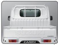
The angle post prevents cargo from banging across the cabin and convenient for tying down cargo with rope.
