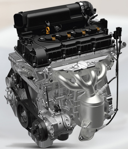
1.2L Engine Displacement: 1,197cc Max Output: 82hp @ 6,000rpm Max Torque: 113Nm @ 4,200rpm
