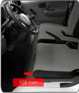
A sliding seat mechanism allows driver to adjust the seat for a comfortable driving position. The seat can be moved a total of 105mm
